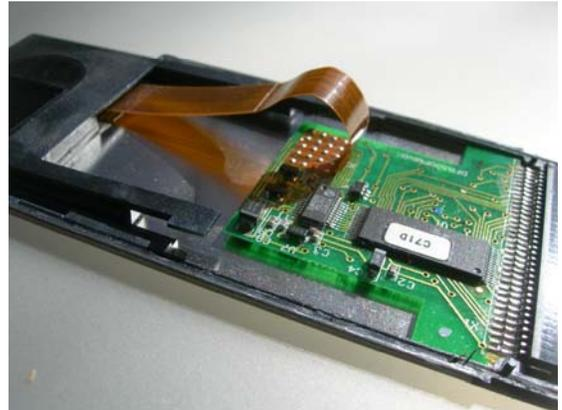
During reliability testing, it was discovered that PCB process could cause wear and tear or binding.
