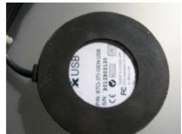
The use of metalized plastic offered a grounding effect for the expected electrostatic discharges. A beautiful and elegant solution to a small EMI generator.
