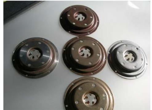
Customer's requirements for the five center fingers for interfacing with center spool had to be within 0.003" tolerance for co-orbital allowable repeatable run out.
