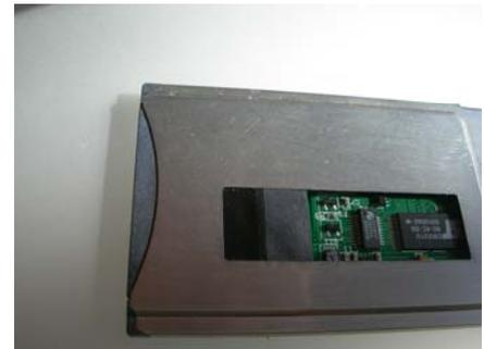
I ordered a windowed test slot during failed units [previously welded closed] to study test failures of the flex circuits and confirmed the "failure mode;" thus a PCB 610 requirement was refined and held as a critical to function inspection point; while the communication flow moved as flowingly as this mechanical design.
