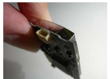
Final lens was hand assembled that fit with precision over the CCD where the optics and interface needed to be aligned.
