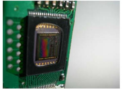
The rainbow pattern, barely seen on the surface is the result of the Fresnel Lens placed on the surface. This is an amazing feat of micro angles curved, focused and reliable from a plastic part. A feat only a optical mold company could perform and a brilliant set of Russian Engineers in St. Petersburg could design. A well executed process by suppliers and inspection fixtures and photo training with optical recognition software as being the final inspection source for focus and occlusions.
